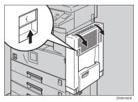
**2** Open the machine's right cover by pushing up the catch.
